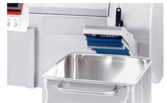
Conveyor belt (above). The outlet (see below) can be regulated and thus ideally adapted to the further process.
